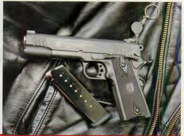
Here the Safety Key is seen inserted into the PT 1911's Safety Lock. When applied, the lock allows the magazine to be removed, but locks the hammer and slide.
